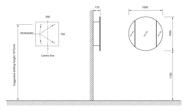
The guide provides a suggested installation height for the Mirage cabinet however please ensure you adjust according to the height of the user and space. The diagram above demonstrates how to install the 800mm Mirage Shaving Cabinet at total height (top of mirror) of 2180mm.
