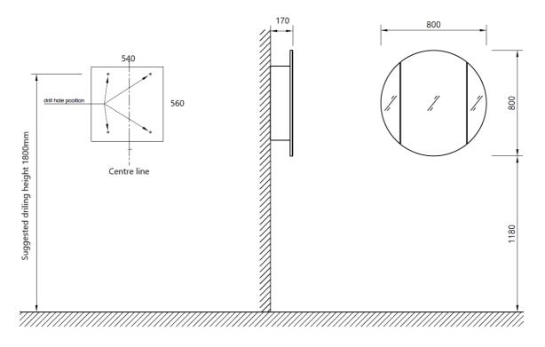
The guide provides a suggested installation height for the Mirage cabinet however please ensure you adjust according to the height of the user and space. The diagram above demonstrates how to install the 800mm Mirage Shaving Cabinet at total height (top of mirror) of 1980mm.
