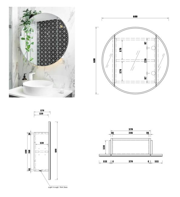
The Mirage Round Mirror Shaving Cabinet embodies the marriage of design and functionality. Available in both a frameless and black trim, this cabinet is ideal for any modern Australian bathroom. Completely recess into your wall for a seamless finish, or semi recess to access the built in undermounted light trough and add to the ambiance of your new bathroom.
