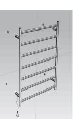
(4)Connect the assembled rail with the fix bases and special fix base in the wall.
