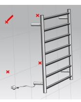
②Mark the desired spot according to the rail dimension , drill holes and install the plastic expanders.
