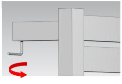
⑤Tighten four legs with M5\*6 Mounting Screw.
