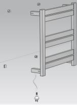
4 Connect the assembled rail with the fix bases and special fix base in the wall.
