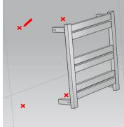
②Mark the desired spot according to the rail dimension, drill holes and install the plastic expanders.
